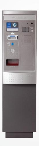
The OPUS-2000 Series Entry Terminal communicates with Pro+ and utilizes an encrypted 2D data matrix barcode for expedited entry to parking facilities. The OPUS-2000 Series offers intuitive user guidance through a dynamic color display and voice announcement. The Entry Terminal dispenses thermal encrypted 2D barcode tickets. Mobile credentials, and printed barcode passes can be processed through the optional FlexScan QR400® barcode scanner.
